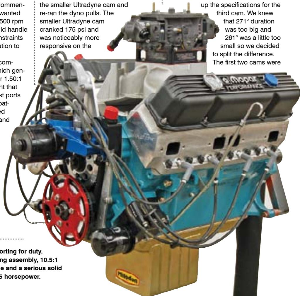
Low deck 470 CID engine reporting for duty. Trick Flow heads, SCAT rotating assembly, 10.5:1 compression, Mopar M1 intake and a serious solid roller camshaft adds up to 685 horsepower.
