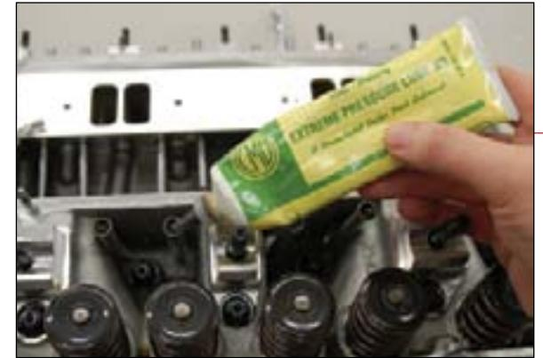
With almost 600 psi of spring force at max lift the pushrod cups see a lot of pressure. Therefore, we put a dab of extreme pressure grease in each cup during assembly. The pushrods have a hole in each end to feed oil directly to the pushrod cup. The direct oil feed keeps the ball and cup fully lubricated when running high spring force.
