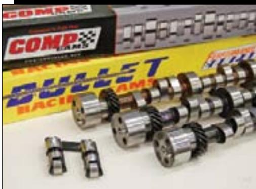
We tested three different solid roller camshafts with fairly classic results. The smallest cam made the most torque while the largest cam had the most peak power. The compromise cam split the difference. In other words, we did not discover free lunch.
