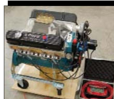
Just for fun the engine was weighed on a chassis scale after dyno testing. Ready to run the 470 weighed 516 pounds which is about 100 pounds lighter than a stock 400.
