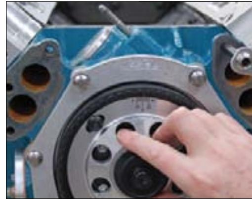
Adjusting the camshaft installed centerline is as easy as loosening up four nuts on the drive wheel and then rotating the cam. The Jesel belt drive is very accurate. If the cam is ground properly the lines on the drive gear will typically agree exactly with the calculated advance or retard figures.
