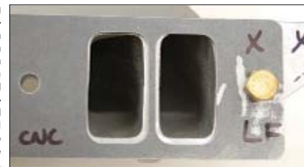
**TOP RIGHT:** We also tested a new Holley 950 which had been converted to annular boosters. The annular boosters increased low speed torque by up to 50 ft-lb when compared to the 850 carb but peak power stayed the same. Annular boosters work really well with cold air and fuels with low vapor pressure since they discharge the fuel through a lot of tiny holes. The downleg booster in the 850 carb works better at higher engine speed and with high RVP fuels.
