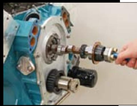
The Jesel belt drive provides for hassle free cam swaps. The oil pan gasket isn't disturbed and the belt is dry. The black flange on the nose of the cam controls the camshaft end play.
