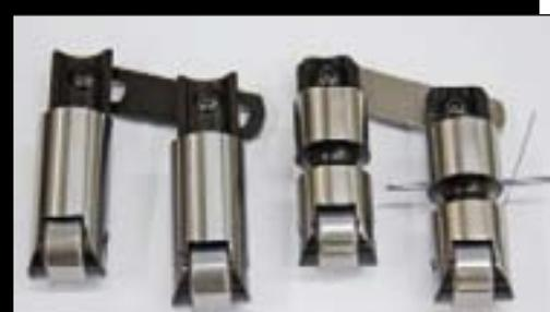
**RIGHT:** One old time hot rodder trick is to use AMC lifters in a Chrysler engine. The AMC lifter on the right has pushrod oiling as well as pin oiling while the standard Chrysler lifter on the left has neither. The AMC lifter is Comp part number 848, the Mopar lifter is a Comp 829.
