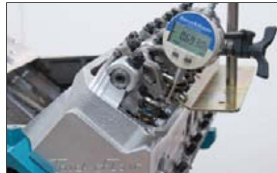
The Bullet cam had 0.460" lobe lift which works out to 0.690" gross lift using 1.50 rocker arms. We're reading 0.693" lift here which means that the rocker arm ratio is a tickle more than 1.50. Not really a problem, but the valve springs are only rated to 0.700 lift so we are getting very close to max travel. Always check for coil bind.
