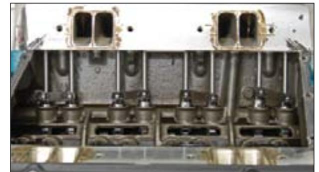
This view of the valley shows the AMC 848 lifters in place using the Comp 829-L link bars. The standard AMC link bars are too long so you have to order individual lifters and then add the Chrysler link bars. Another option is to buy lifters with pushrod oiling capability from Crane or Morel.
