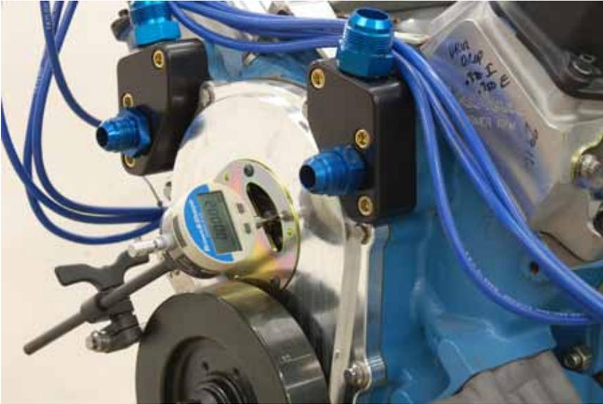
A cover with a slotted opening is provided so the engine builder can easily set camshaft end play. Mount a dial indicator as shown in the picture with the plunger resting on the camshaft nose or the timing gear. Pry the camshaft back and forth and measure the endplay.
