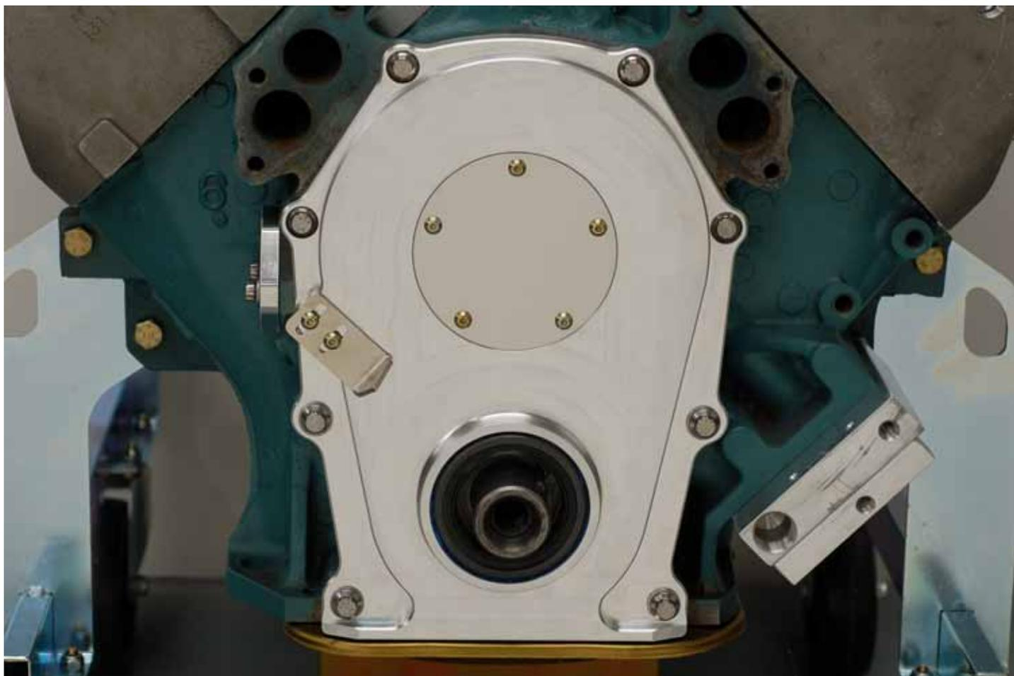
This billet cover will fit under a Mopar Performance aluminum water pump housing without the need for any spacers. A factory cast iron water pump housing will need some minor grinding in order to clear this cover. Meziere water pumps usually fit without any modification. ATI, Fluidampr, OEM and BHJ dampers all fit this cover without any modifications.
