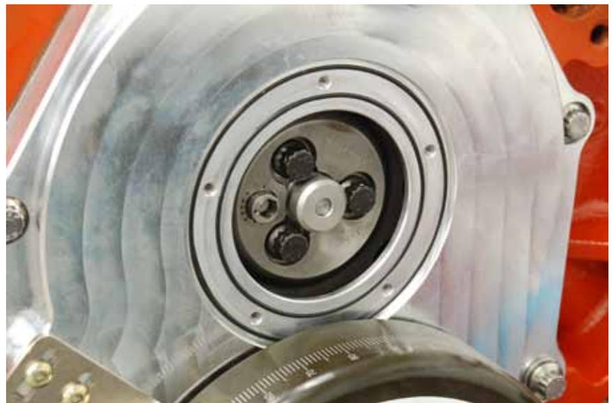
The endplay specification is typically 0.005 to 0.010 inches for most camshafts. The AR281 button is designed to have 0.010 inches of endplay when used with a 0.032 thick timing chain gasket. Timing chain gaskets are available from Superformance Products in thicknesses ranging from 0.022 to 0.062.
