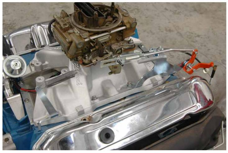
This throttle bracket is designed to work with an Edelbrock Performer RPM manifold on a big block engine. There are two versions of this bracket, AR036 fits the 383/400 engine family while AR018 fits the 413/426/440 family. The bracket is the correct height to allow you to connect a factory three section throttle rod to a factory carburetor when using the taller Edelbrock manifold.
