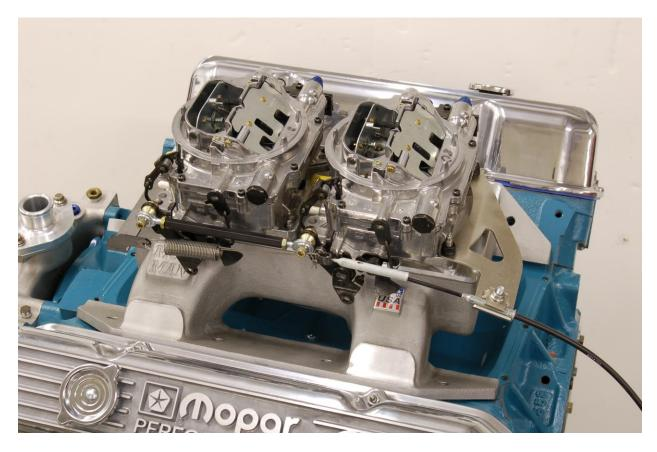
This throttle linkage kit is designed to work with Edelbrock Performer style carburetors on the Indy ModMan dual 4bbl intake. The linkage kit uses Heim joints on each end to avoid binding and to allow maximum adjustability.
