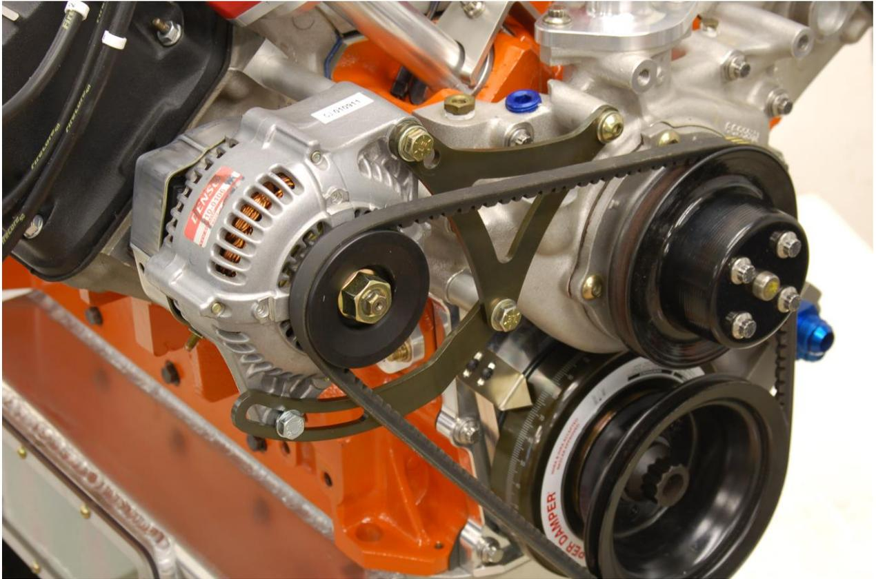
This kit contains the mounting brackets, spacers and bolts necessary to adapt a lightweight Denso alternator from a Toyota 4Runner (1985 to 1991 with L4 engine) to a Chrysler 426 Hemi engine. The kit contains two aluminum spacers, as well as upper and lower mounting brackets and three mounting bolts. This kit works with the Hemi water pump pulley set shown in the picture (Mopar Performance number P4510282). The lower pulley needs to be a matching Hemi pulley.
