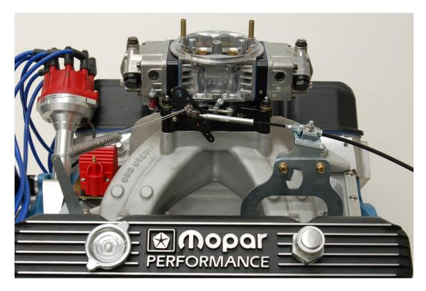
This throttle bracket kit provides proper alignment for the throttle cable on a high rise manifold. A big block kit is shown above, but kits are available for small block (LA, W2 and Magnum), big block (B and RB), and street Hemi manifolds. The operation of the bracket is the same for either application.
