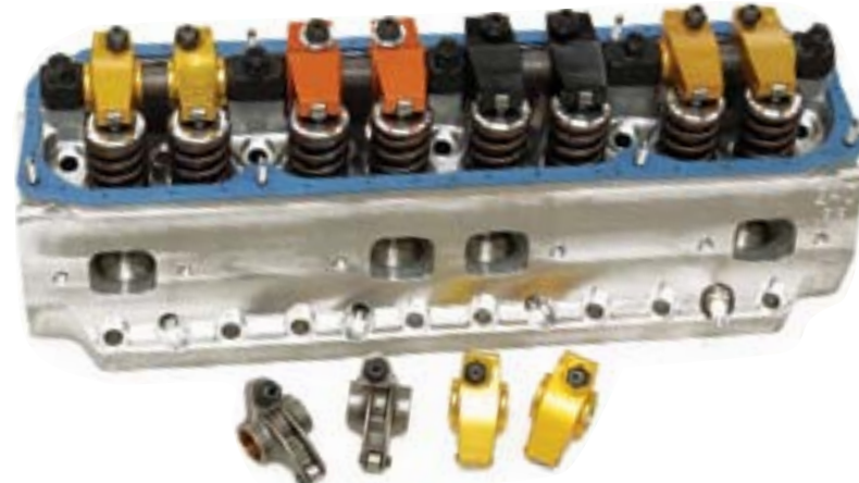
The rocker shaft is relocated higher on the Trick Flow heads by roughly 5/8-inch in order to provide more room for longer valves and valve springs. We took a quick look at the resultant geometry with various rocker arms and came to the conclusion that the shorter rocker arms such as those from Crane (right) and Comp (l.) would be our first choice.
