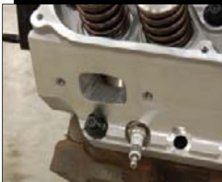
The ports on the Trick Flow head are fully CNC machined. This view of the exhaust port shows the fairly large step over that Trick Flow uses in their CNC machining. The spark plugs are angled similar to Edelbrock or Indy heads.
