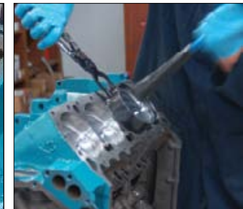
Once the crankshaft is fully secure the piston and rods can be knocked into place using a ring compressor and plenty of lube. Of course a bore-specific ring compressor, or even the wrinkle-band type, makes this job easier.
