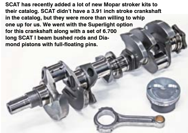
The SCAT Superlight crankshaft only weighs 54 lbs. so it is easy to drop in place. We used an ARP main stud kit to provide a little extra clamping force on the main caps.
