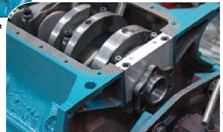
ABOVE: A close up of the SCAT Superlight crankshaft shows the fully machined counterweights as well as the gun drilled mains and the hollow rod journals.
