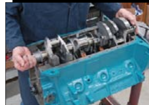
The SCAT Superlight crankshaft only weighs 54 lbs. so it is easy to drop in place. We used an ARP main stud kit to provide a little extra clamping force on the main caps.
