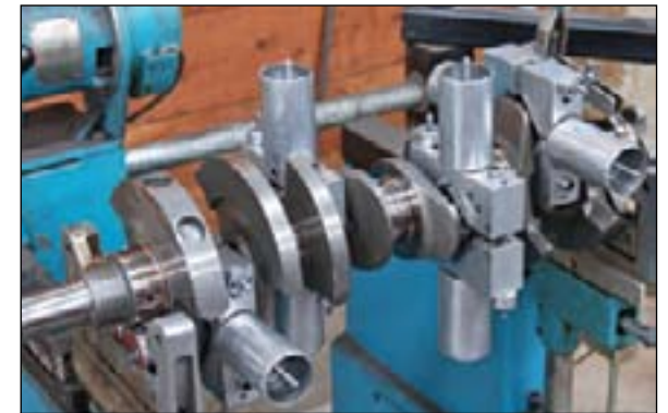
The SCAT Superlight crank is rough balanced but we needed to dial it in once we had all of the other parts. Finished bobweight for this rotating assembly is only 2222 grams - over a pound lighter than an OEM 440!
