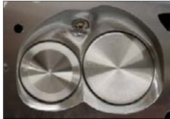
The combustion chamber in the Trick Flow heads is fully CNC machined with a finished volume of 78 cc. The intake valve is 2.19 inches while the exhaust is 1.76 inches.
