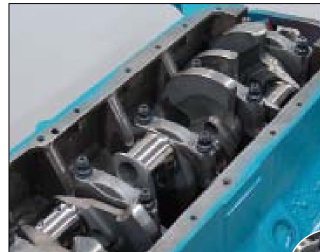
ABOVE: A close up of the SCAT Superlight crankshaft shows the fully machined counterweights as well as the gun drilled mains and the hollow rod journals.
