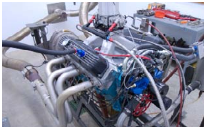
The 470 low-deck alive and on the dyno! We were able to get a handful of shake-down runs on the new engine before this article went to press and we're happy to say that we've seen 590 ft-lbs of torque and 660 hp. We expect those numbers to increase as we get the new combination tweaked and sorted out.
