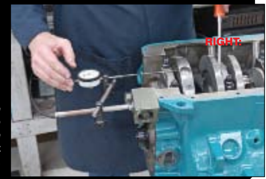
The SCAT Superlight crankshaft only weighs 54 lbs. so it is easy to drop in place. We used an ARP main stud kit to provide a little extra clamping force on the main caps.
